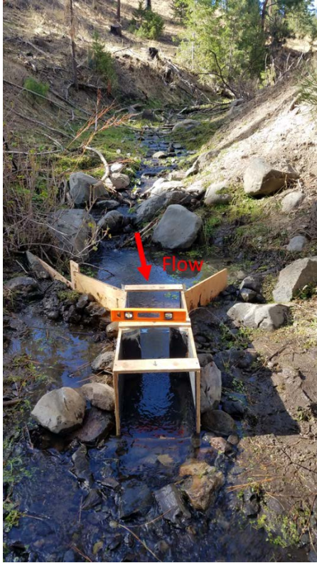
Streamflow measuring device installed at the outlet of Fish Creek.
