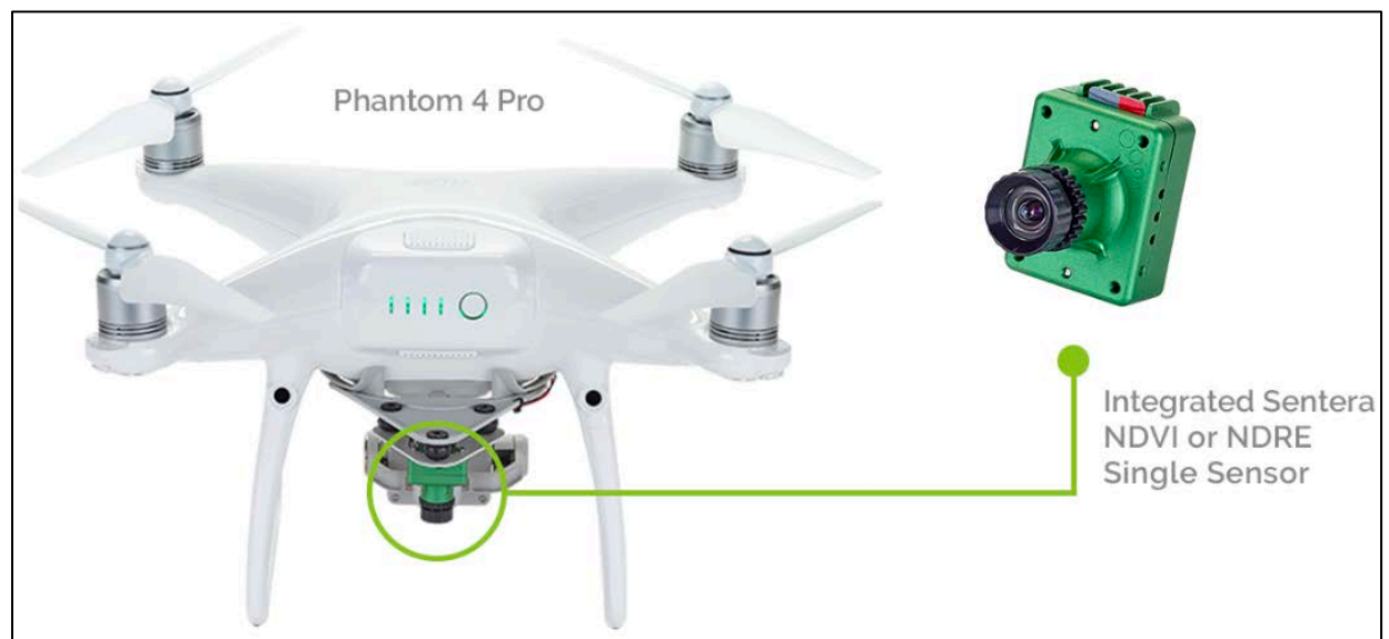
Figure 1: This project will utilize a DJI Phantom 4 Pro drone with a Sentera NDVI single sensor.
